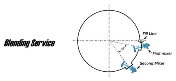
Locating the mixer(s) approximately 15 degrees to the left of the Fill Line compliments mixer performance and encourages product to be pulled into the mixer propeller and quickly dispersed into the tank.
