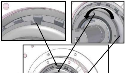
9. Partially thread in 1/4-20 bolts (shown with arrows) to aid in turning RETAINING RING with screwdriver.
