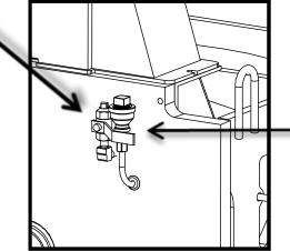
Leak Detection Inlet
