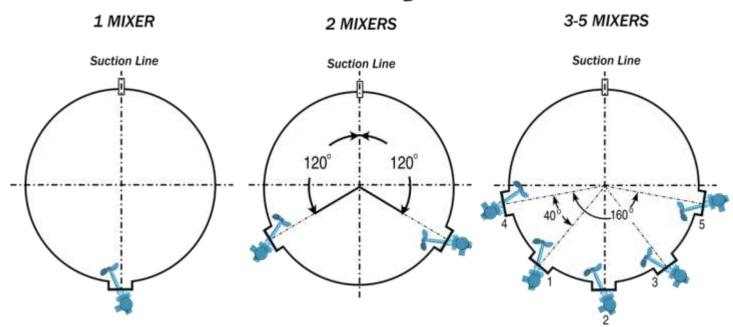
Locating the mixer(s) at the opposite side of the Suction Line the allows the user to take advantage of the natural cleaning that will occur due to product being drawn from the tank.
