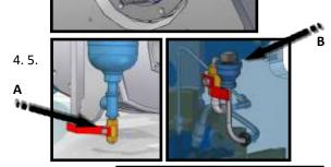
6. Remove SHAFT BOLT (¾ OPEN WRENCH), YOKE, and KEY
