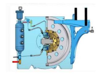
MECHANICAL SEAL stationary pin should be in contact with either anti-rotation pins located at the 3 or 9 O'clock position in the seal chamber.
